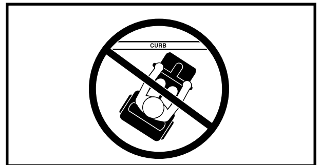
Figure 7. Incorrect Curb Approach
