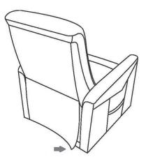
10. Place the chair in the desired position in the room, keeping it 21" away from the wall. If placing the chair into a corner, keep it 21" from the wall as shown. See distance chart below for your model.
