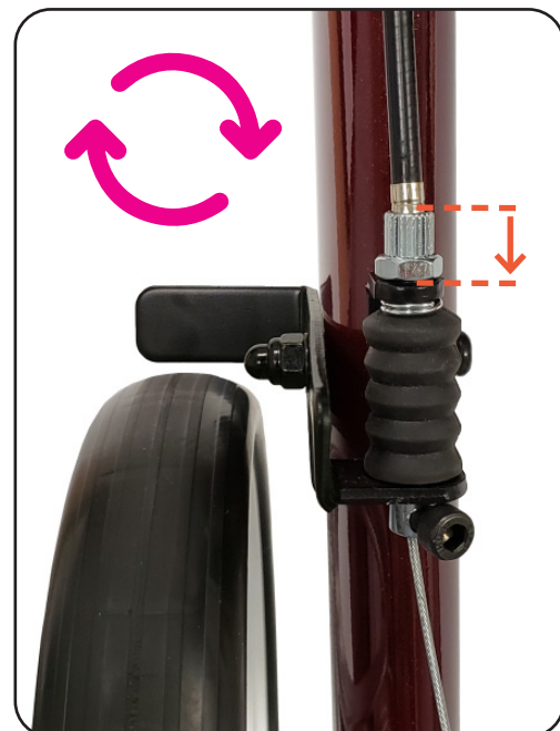
Loosen the Brake
